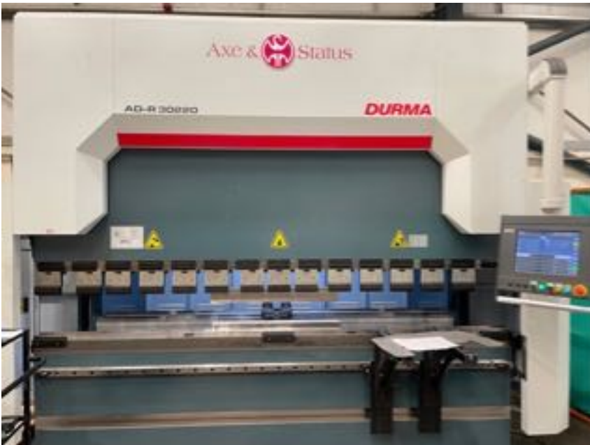
225-ton CNC Press brake for steel bending up to 3 meters wide.
