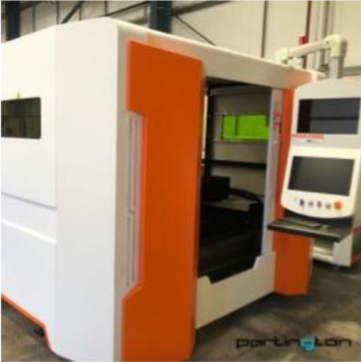
3KW laser that can cut mild steel up to 16mm and stainless steel up to 12mm
