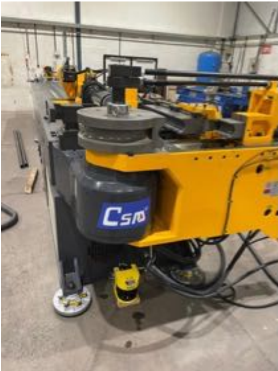
CNC tube bender that can form tube from 16mm diameter to 101mm diameter
